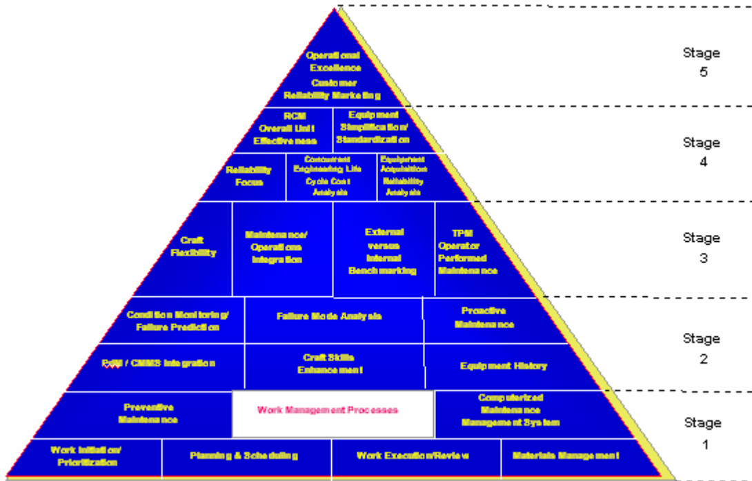
Figure 2: Stages of Maintenance Excellence
